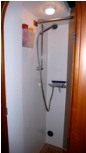
Adjacent is a roomy dedicated shower cabin with a teak grated two-piece teak sole equipped with thermostatically controlled shower taps. An opening deck hatch provides ventilation.
