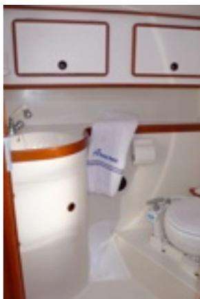
Opposite, to starboard of the centerline companionway, is the head compartment, finished in white laminate with varnished teak trim. A Jabsco head is aft, a hand washbasin with mixer and shower tap is let into the vanity outboard. Light and air are provided by one opening deck hatch.
